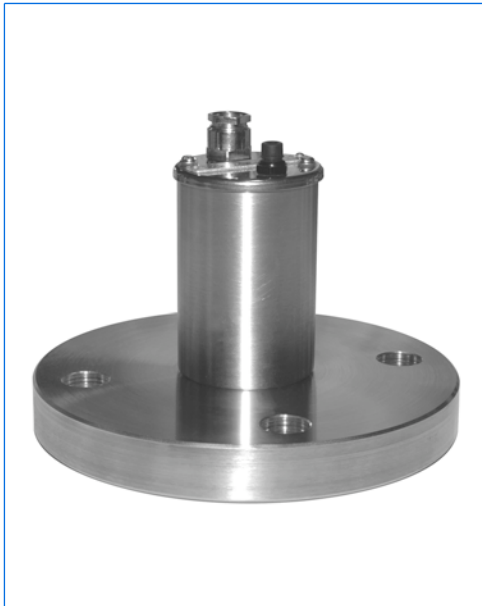
Light fitting miniLUX STERI-LINE, type BKVLR 20 HDA, 20 W, 24 V, mounted on a metal fused sightglass flange for sterile applications, DN 50
