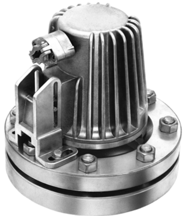
Type F 20 dHSchU, Ex d IIC T5 Gb, Ex t IIC T95°C Db IP67, Ex II 2 G + D, halogen bulb, 230 V, 20 W, with built-in timer «U», mounted on sightglass to DIN 28120, DN 125, PN 10, with tilting hinge fixation "Sch"
