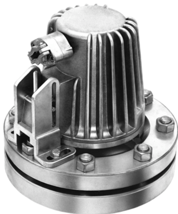
Type F 20 dHSchU, Ex d IIC T5, Ex tD A21 IP65 T95°C, Ex II 2 G + D, halogen bulb, 230 V, 20 W, with built-in timer «U», mounted on sightglass to DIN 28120, DN 125, PN 10, with tilting hinge fixation "Sch"
