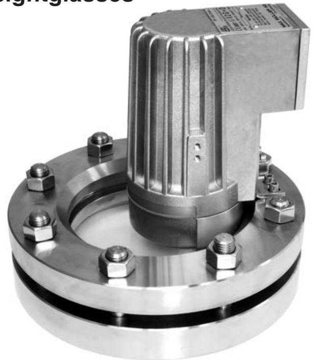
Type HEL 50 deHW, Ex d e IIC T3 Gb, Ex t IIIC T195°C Db / IP67, Ex II 2 G + D, 230 V, 50 W, halogen version, mounted on circular sightglass to DIN 28120, DN 125, PN 10, in 1 port version.
