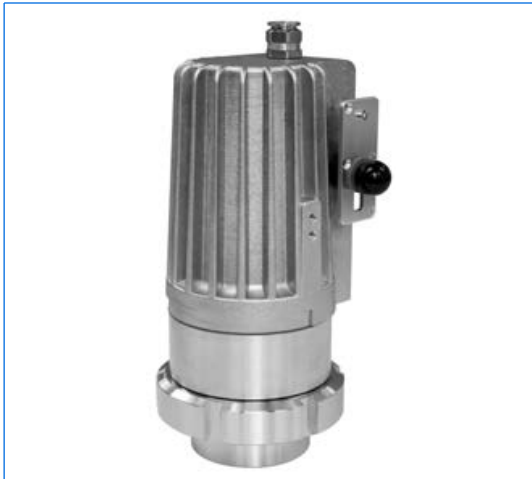
Type FHEL 35 dHVRK1, Ex d IIC T4 Gb, Ex t IIIC T130°C Db / IP67, Ex II 2 G + D, 230 V, 35 W, halogen version, with timer "V", on screwed sightglass similar to DIN 11851, DN 65, PN 6. Fixation with intermediate flange collar "R".
