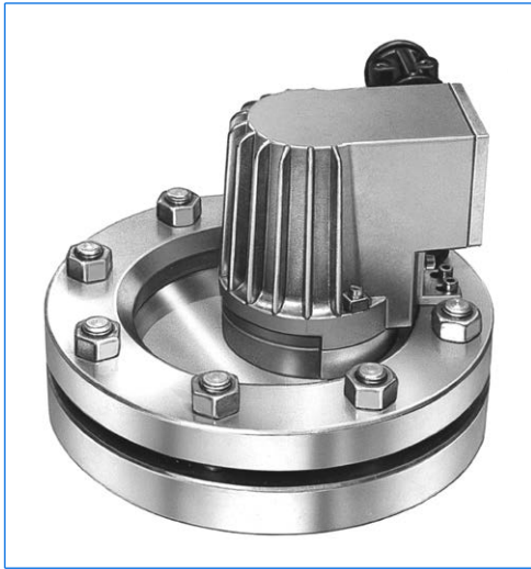
Hazardous area type KEL de PowerLED W, Ex de op is IIC T6 Gb, Ex tb IIIC T80°C Db, IP65/67, Ex II 2 G + D, 230–240 V AC, 7 W, mounted on circular sightglass to DIN 28120, DN 125, PN 10, in 1 port version.
