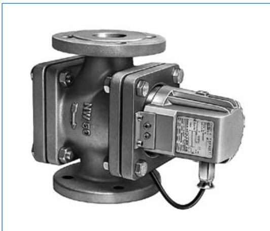
Hazardous area type FKEL 5 dH WM, Ex t IIC T6 Gb, Ex t IIC T80°C Db IP67, Ex II 2 G + D, 230 V, 5 W, with opal glass "M", on pipeline flow indicator DN 50.
