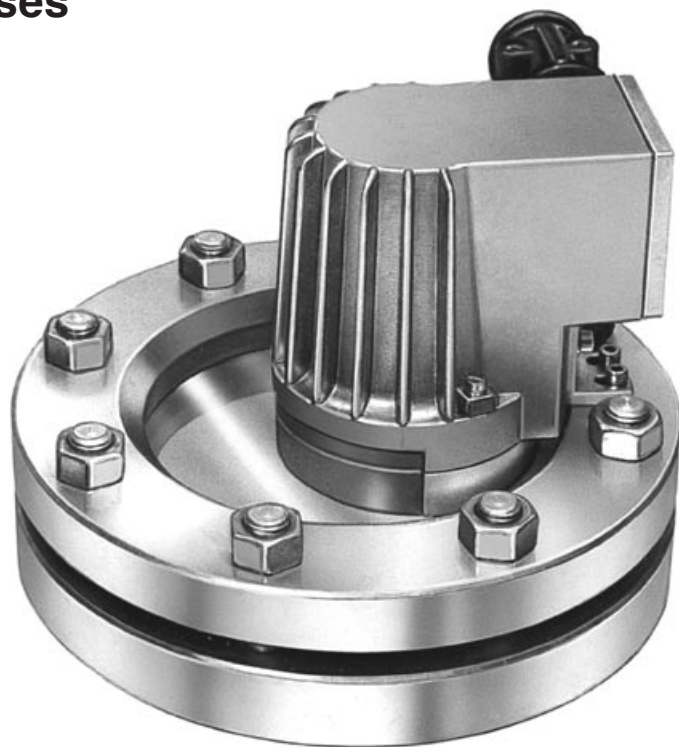
Type KEL 20 deH W , Ex de IIC T4, Ex tD A21 IP65 T130°C, Ex II 2 G + D, 230 V, 20 W, mounted on circular sightglass to DIN 28120, DN 125, PN 10, in 1 port version.
