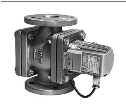
Hazardous area type FKEL 5 dH WM, Ex d IIC T6, Ex tD A21 IP65 T80°C, Ex II 2 G + D, 230 V, 5 W, with opal glass "M", on pipeline flow indicator DN 50.
