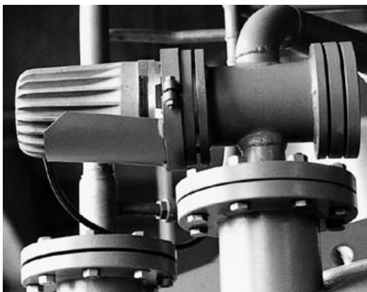
CHEMLUX ® sightglass light fitting, type L 20 deH sp, 20 W, 24 V, Ex de IIC T5, Ex tD A21 IP65 T95°C, Ex II 2 G + D, mounted with an opal glass screen "M" on a pipeline flow indicator
