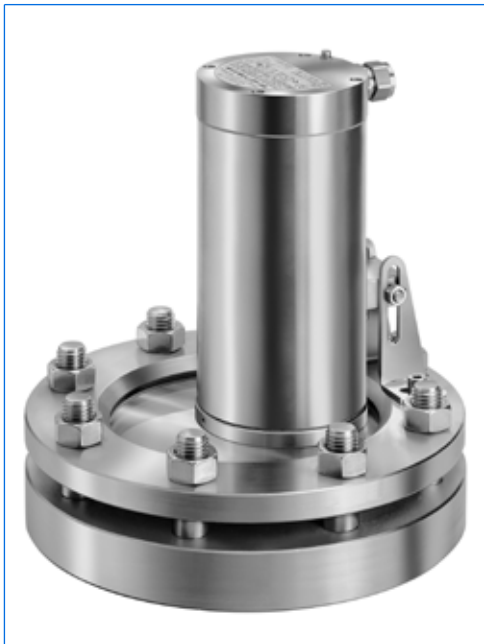
Sightglass light fitting type EdelEx 50 dH Sch K2, 50 W, 230 V, Ex d IIC T4, Ex tD A21 IP65 T130°C, Ex II 2 G + D, mounted on circular sightglass to DIN 28120, PN 10, DN 150.
