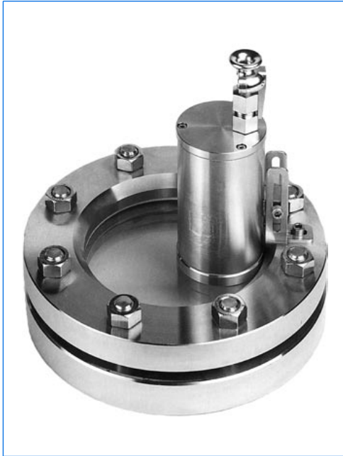
Sightglass light fitting type EdelEx d LED Sch K1, ca. 5 W, 100 - 240 V, Ex d IIC T6, Ex tD A21 IP65 T80°C, Ex II 2 G + D, mounted onto circular sightglass to DIN 28120, PN 10, DN 125.
