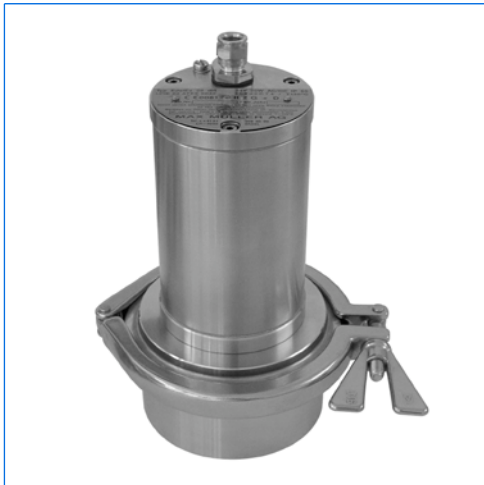
EdelLUX LED sightglass light fitting, type EdelEx LED, Ex d II C T6, Ex tD A21 IP 65 T80°C, Ex II G + D, mounted onto metal fused sightglass for Triclamp® fittings, DN 50, PN 16
