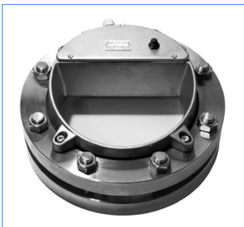
metaLUX LED sightglass light fitting, type HL 200 LED, on sightglass to DIN 2810, DN 200, PN 10
