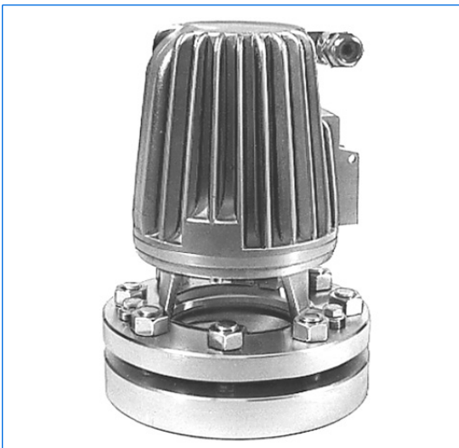
VETROLUX illuminated sightglass unit, consisting of sightglass to DIN 28120, DN 80, PN 10, with mounted CHEMLUX light fitting, type F 20dHNsp, 24 V, 20 W, Ex d IIC T5 Gb, Ex t IIIC T95°C Db IP 67, Ex II 2 G + D
