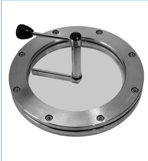
Circular sightglass, DN 150, PN 0, with glass disc in sodium silicate to DIN 8902 and wiper of the series W, wiper blade in silicone
