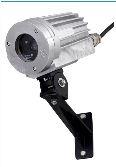
Ex camera miniZoom, aluminium alloy enclosure, Ex d IIC T6, Ex tD A21 IP67 T80°C, Ex II 2 G + D, with wall fixing system.
