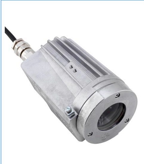
Ex camera miniZoom, aluminium alloy enclosure, Ex d IIC T6, Ex tD A21 IP67 T80°C, Ex II 2 G + D.
