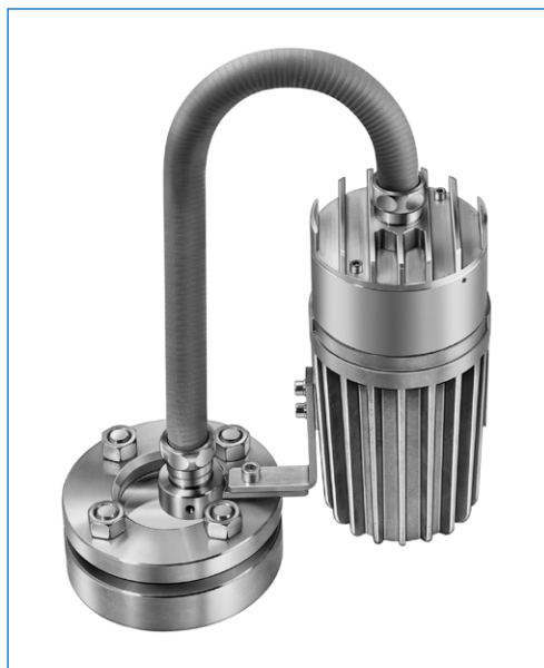
Fibre-optic lightpipe light fitting with built-in timer "U", type fibroLUX® 5035 W W2 U sp, Ex de IIC T4, Ex tD A21 IP65 T130°C, Ex II 2 G + D, 35 W, 12 V DC, fixation of the light source by bracket "W", fixation of the lightpipe by universal support "W2" onto sightglass to DIN 28120, DN 40, PN 10
