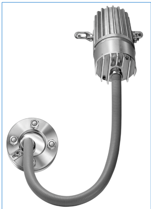
Fibre-optic lightpipe light fitting for use in hazardous areas with built-in timer "V", type fibroLUX® 5035 X1 W2 V, Ex de IIC T4, Ex tD A21 IP65 T130°C, Ex II 2 G + D, 35W, 230V, fixation of the light source by fixation legs "X1", fixation of the lightpipe by universal support "W2" onto sightglass to DIN 28120, DN 40, PN 10
