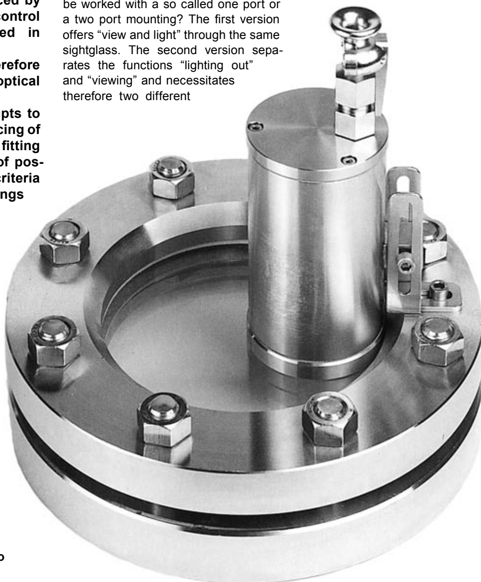
Fig.1 EdelLUX® light fitting type EdelEx, completely in stainless steel, 20 W, 24 V, Ex d IIC T4, Ex tD A21 IP65 T130°C, Ex II 2 G + D, mounted on a VETROLUX® sightglass to DIN 28120
