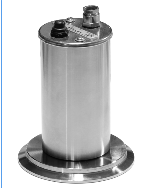
Sightglass light fitting type KLR 20 HDA Sp, 20 W, 115 V, with built-in momentary push-button "D", on metal fused sightglass for Triclamp fittings, DN 100
