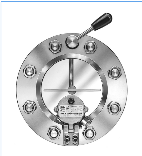
Wiper system WS, built into a VETROLUX® sight-glass to DIN 28120, DN 100, PN 10, with mounted sightglass light fitting miniLUX®, type KVL 50 HDSch, 24 V, 50 W, for combined “view and light through one assembly”.
