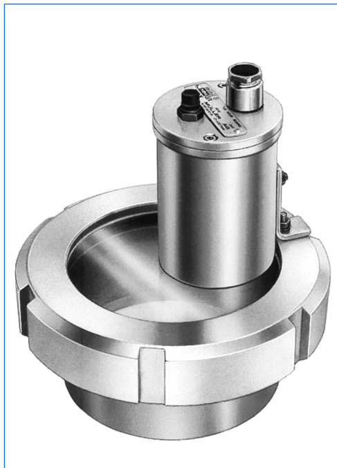
Sightglass light fitting type KVLR 50 HDW1, 50 W, 24 V, with built-in momentary push-button "D", mounted by bracket "W1" on screwed sightglass similar to DIN 11851, DN 100, PN 6, for application "view and light through one assembly".
