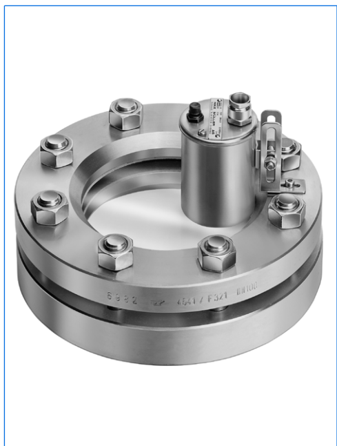
Sightglass light fitting type BKVLR LED DSch, 24 V, with built-in momentary push-button "D", mounted with tilting hinge "Sch" on sightglass to DIN 28120, DN 100, PN 10, for application "view and light through one assembly".
