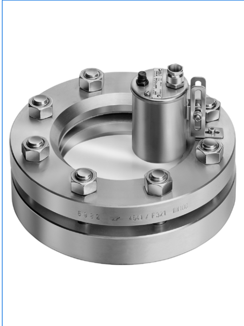
Sightglass light fitting type BKVLR 20 HDSch, 20 W, 24 V, with built-in momentary push-button "D", mounted with tilting hinge "Sch" on sightglass to DIN 28120, DN 100, PN 10, for application "view and light through one assembly".
